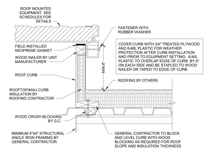
NOTE: 1. ROOF FLASHING AND COUNTERFLASHING NOT SHOWN FOR CLARITY AS THESE ELEMENTS WILL BE FURNISHED AND INSTALLED BY THE ROOFING CONTRACTOR
